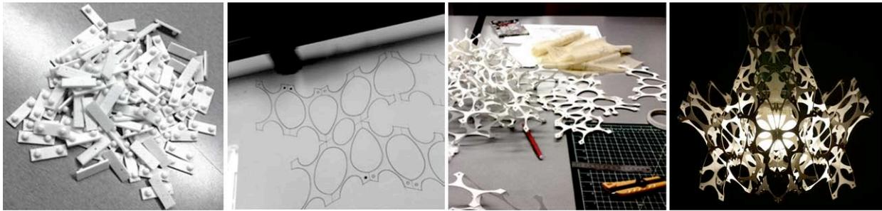
Fig. 1: (Left to Right) 3D prints of connection pieces, laser cutting of frames, assemblage of elements, and final light
