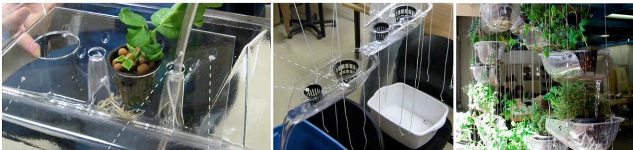
Fig. 3: (Left to Right) A sample of iterations of a hydroponic irrigation system over the course of a month from an initial vacuum formed tray configuration, to a basket configuration, to a fully secured assembly
