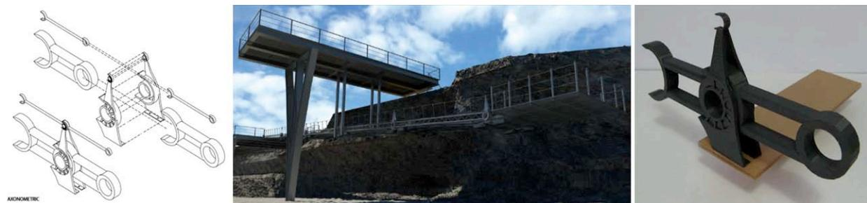
Fig. 2: (Left to Right) A CAD model of the detail, a rendered view of the connection in context, and an operable developmental prototype from the 3D printer used for design development of the hinge
